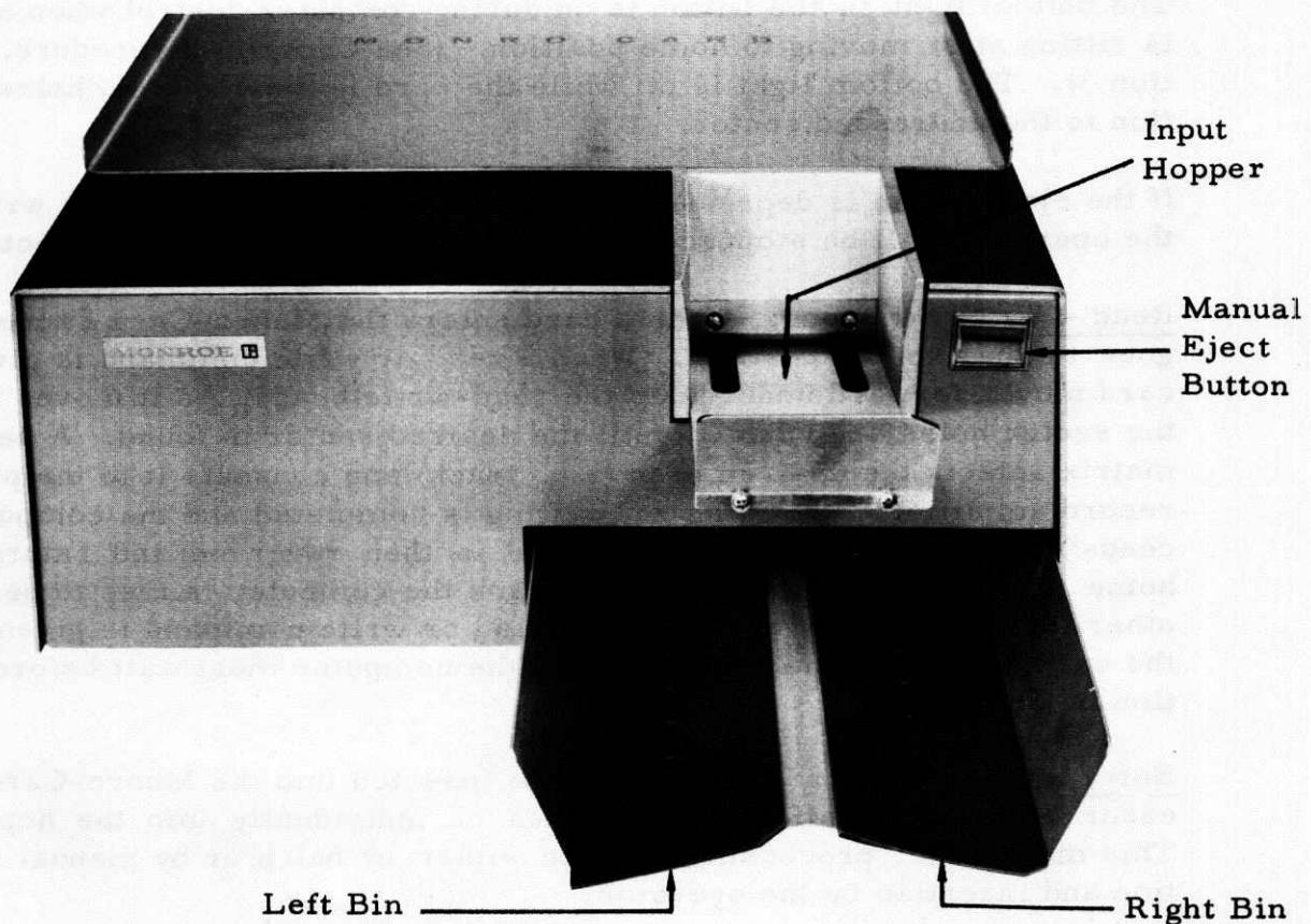
Input Hopper: Cards are placed in the input hopper with the magnetic oxide coating (the brown side) up and with the cut corner away from the card unit. A small weight is supplied which should be placed on top of stack of cards to assure that the cards are fed properly. The bottom card (the first one
